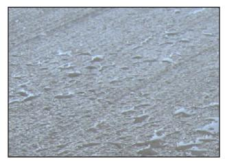
Water is applied over CLEAR SEAL WB 3 hours after initial application. This broom finished concrete surface demonstrates the early water resistance properties that develop with the CLEAR SEAL WB sealer.
